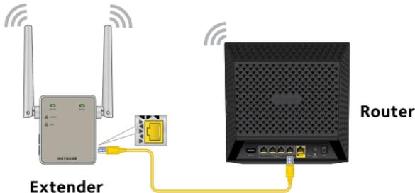
1. Plug the extender into an electrical outlet and wait for the Power LED to light green.
