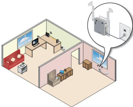
1. Plug an extender into an electrical outlet.
