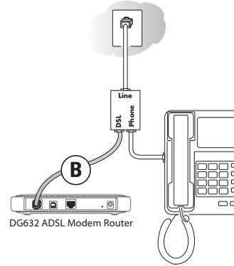
**Note:** Improperly connecting a filter to your DG632 will block ADSL signals and prevent connecting to the Internet.
