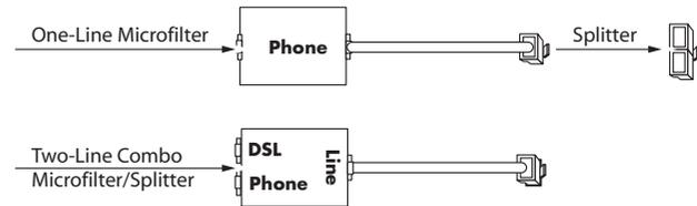
The procedure below illustrates using a two-line combo microfilter/splitter. You can accomplish the same result using a one-line microfilter with a separate phone line splitter.
