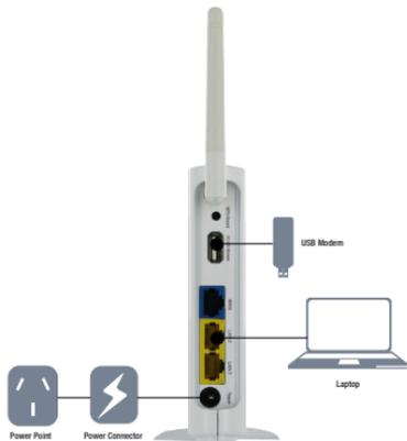
1. With the supplied **Ethernet cable**, connect your computer to one of the **yellow LAN** ports on the back of the 3G17Wn.
