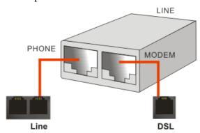
For second WAN, connect the cable Modem/DSL Modem/Media Converter to WAN2 port of router with Ethernet cable (RJ-45).
