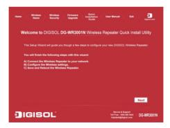
Connect one end of the network cable to the LAN port on the repeater and the other end to the PC's Ethernet port. Power on the repeater and ensure that all the LED's on the repeater are on. Click 'Next' to continue.
