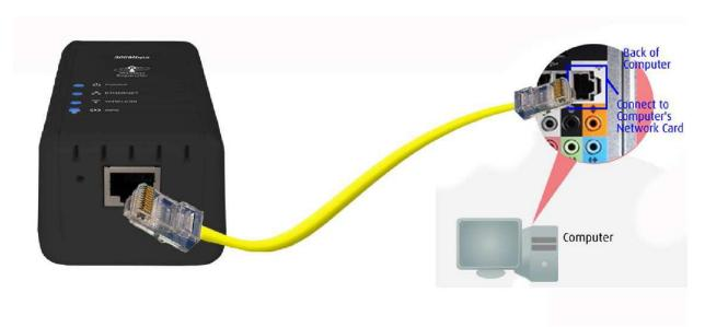
**3.** Once a connection to the WR300N is established, your PC/laptop will receive an IP address and you can start the configuration using the web graphical user interface.
