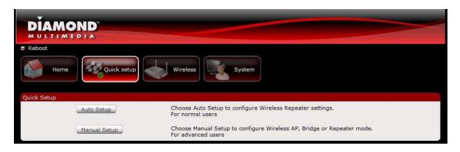
NOTE: If you are connecting to a hidden wireless network, you need to go through the Manual Setup and key-in the information from your existing wireless router/AP manually. Uncheck the broadcast SSID option so that your wireless network will remain hidden.
