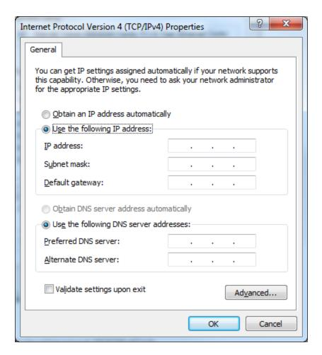
Make sure you select "Use the following IP address" option and enter 10.0.10.1 for the IP address.
