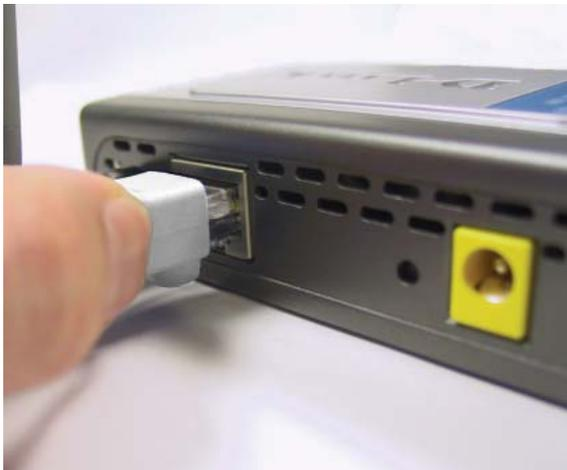
The Ethernet port on the DWL-G820 is Auto MDI/MDI-X. Meaning you can use a straight-through or crossover cable to the Ethernet Port.
