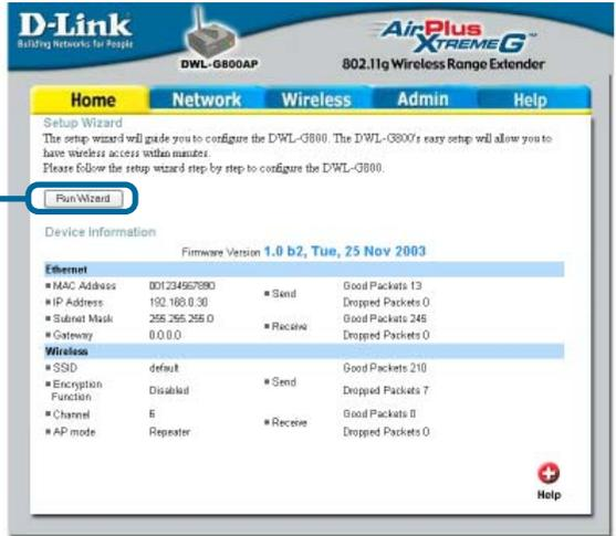
The screenshot shows the D-Link DWL-G800AP Home screen. The top navigation bar includes 'Home', 'Network', 'Wireless', 'Admin', and 'Help'. The 'Home' tab is selected. Below the navigation bar, there is a 'Setup Wizard' section with a 'Run Wizard' button. A callout box points to this button with the text 'Click Run Wizard'. Below the 'Run Wizard' button, there is a 'Device Information' section with a table of statistics for Ethernet and Wireless.
