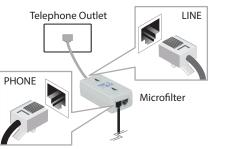
Connect the Phone cable from the DSL port on the Microfilter to the ADSL port of the modem router.
