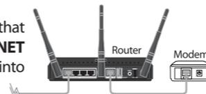
**Step 5** - Reconnect the power adapter to your cable or DSL broadband modem and wait for two minutes.
