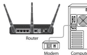
**Step 3** - Unplug the Ethernet cable from your modem (or existing router if upgrading) that is connected to your computer. Plug it into the blue port labeled **1** on the back of your router. The router is now connected to your computer.
