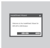
**Note:** You have to install the Connection Manager software when using the DIR-457U for the first time. After successful installation, you can configure USB modem and WiFi router basic settings. Only USB modem mode serves as Connection Manager mode.
