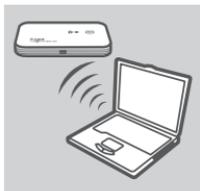
3. You can now use the DIR-457U myPocket Router as a wireless access point and connect to the router with any WiFi capable device.
