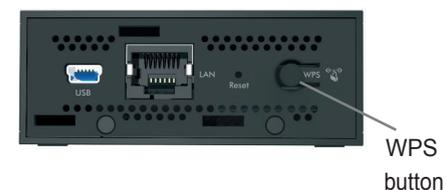
**Step 3:** Push the WPS button on your router. When the wireless connection has been established, the LED changes color to indicate the quality of the connection—solid green, solid amber, or solid red. Check "Adapter LED Activity" on the reverse side for more information about what these colors mean.
