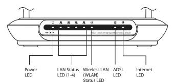
1.6 Turn on your computers. After your computers boot up, a LAN status LED on the front of the Router will light for each port to which a wired computer is connected. These LEDs indicate connection and activity status. Now you are ready to configure the Router for ADSL connection.
