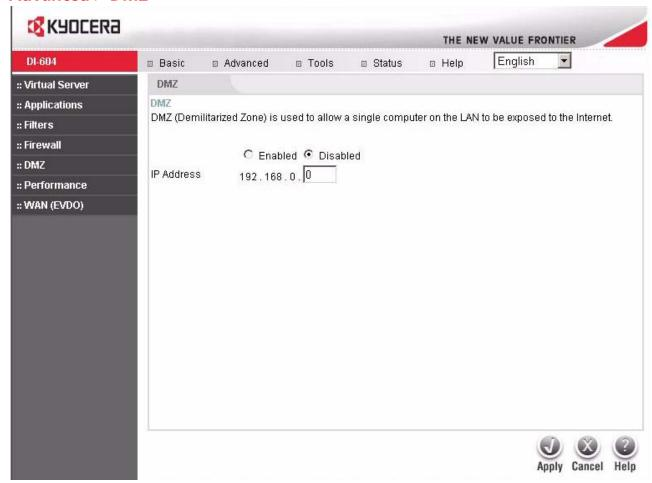
If you have a client PC that cannot run Internet applications properly from behind the Kyocera KR1 Mobile Router, then you can set the client up for unrestricted Internet access. It allows a computer to be exposed to the Internet. This feature is useful for gaming purposes. Enter the IP address of the internal computer that will be the DMZ host. Adding a client to the DMZ (Demilitarized Zone) may expose your local network to a variety of security risks, so only use this option as a last resort.
