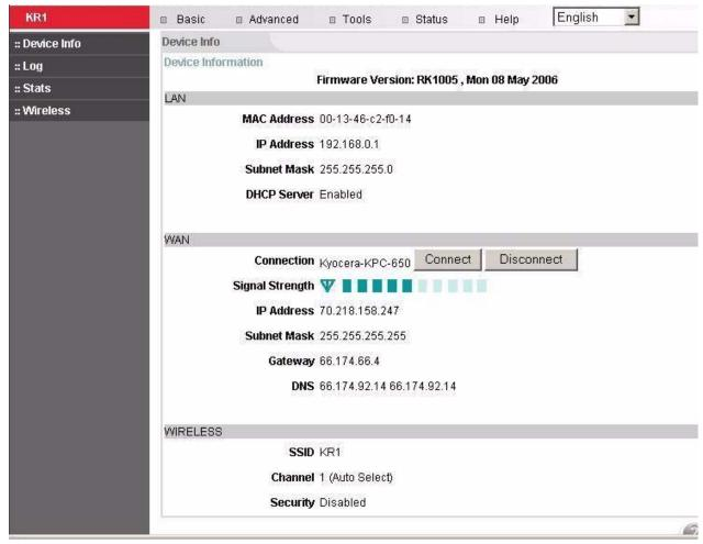
This page displays the current LAN, WWAN, and WIRELESS information for the Kyocera KR1 Mobile Router. A connection to the EVDO network will be established when the unit is powered on. Use the **Disconnect** button to disconnect from the EVDO network; use the **Connect** button to establish a connection.
