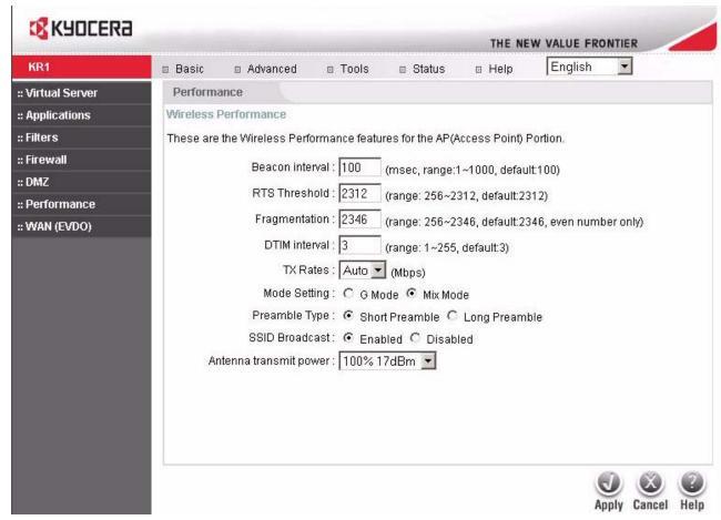
**Wireless Performance-** Displayed in this window are the Wireless Performance features for the Access Point portion of the Kyocera KR1 Mobile Router.
