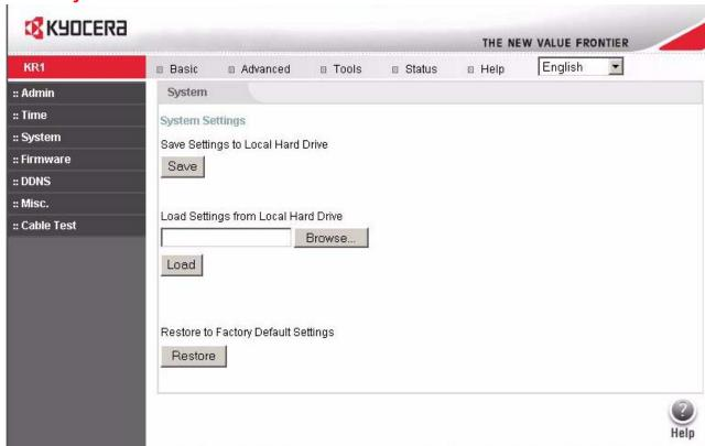
The current system settings can be saved as a file onto the local hard drive. The saved file, or any other saved settings file, can be loaded back on the Broadband Router. To reload a system settings file, click on **Browse** to browse the local hard drive and locate the system file to be used. You may also reset the Broadband Router back to factory settings by clicking **Restore**.
