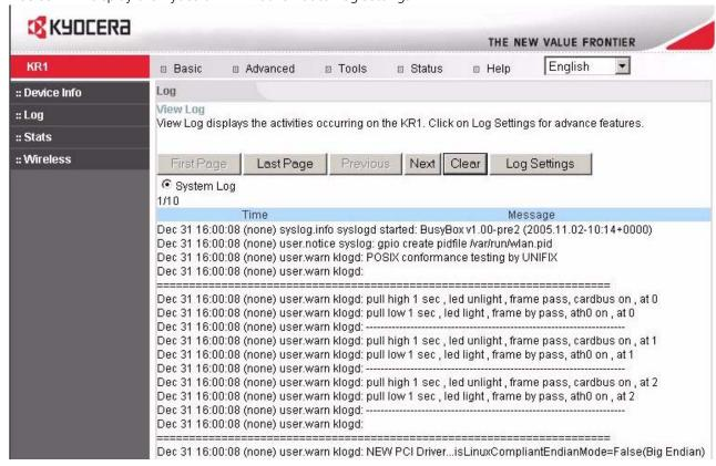
**Note:** If the device is rebooted, the logs are automatically cleared.
