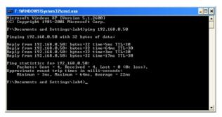
**Note:** If you have changed the **default** IP Address, ensure you ping the correct IP Address assigned to the Kyocera KR1 Mobile Router.
