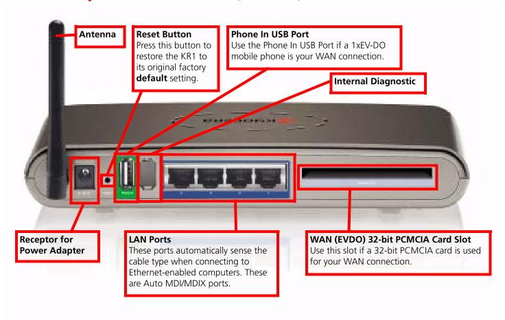
**Note:** The Kyocera KR1 Mobile Router contains two ports: a "Phone-In" USB Port, and a second internal diagnostic port. Please use *only* the "Phone In" USB port for your 1xEV-DO WAN connections. The second port is not for customer use. Please do not attempt to use this port.
