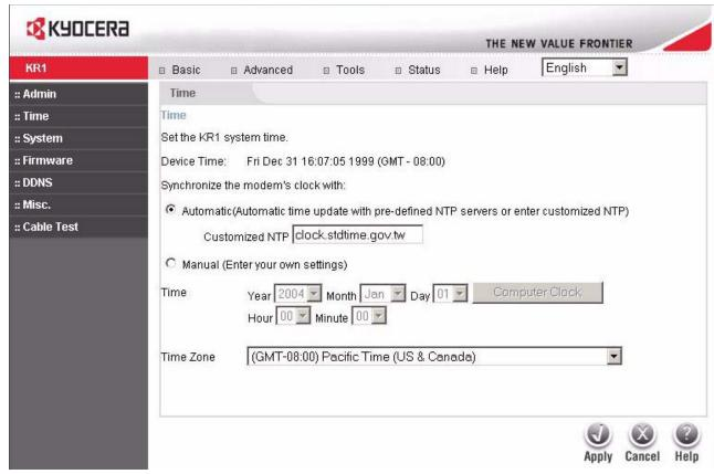
**Synchronize the modem's clock with-** NTP is short for Network Time Protocol. NTP synchronizes computer clock times in a network of computers. You have the option to manually set the time or have it automatically done for you. By **default** the Synchronize the modem's clock with is **Automatic**.
