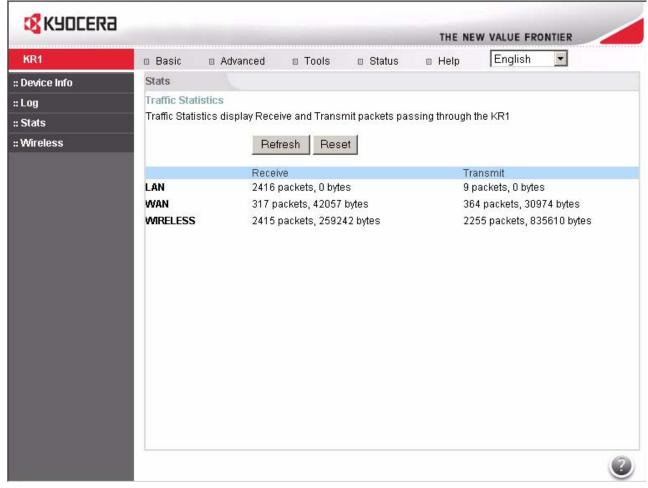
The screen above displays the Traffic Statistics. Here you can view the amount of packets that pass through the Kyocera KR1 Mobile Router on both the WAN and the LAN Ports. The traffic counter resets if the device is rebooted.
