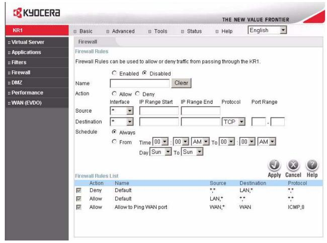
**Firewall Rules** is an advanced feature used to deny or allow traffic from passing through the Kyocera KR1 Mobile Router. It works in the same way as IP Filters with additional settings. You can create more detailed access rules for the Kyocera KR1 Mobile Router. When virtual services are created and enabled, it also displays in Firewall Rules. Firewall Rules contain all network firewall rules pertaining to IP (Internet Protocol).
