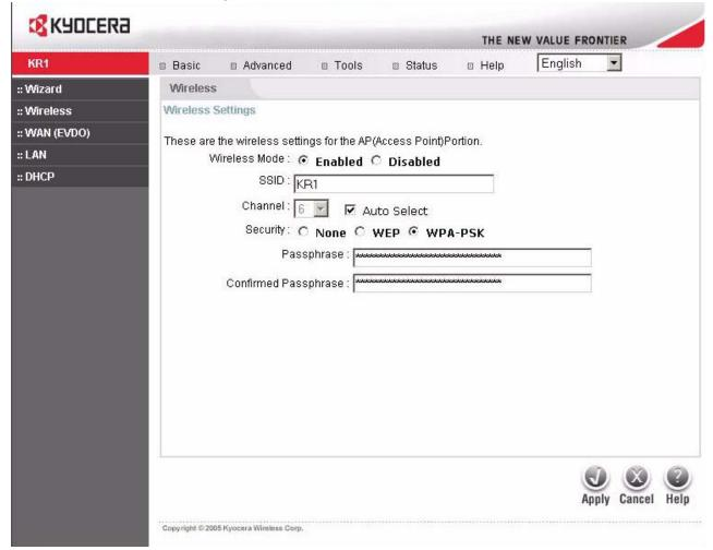
**Security- WPA-PSK-** WPA-PSK authenticates users based on a Passphrase. The default setting does not contain a
