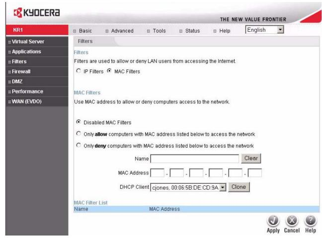
Use **MAC** (Media Access Control) Filters to allow or deny LAN (Local Area Network) computers by their MAC addresses from accessing the Network. You can either manually add a MAC address or select the MAC address from the list of clients that are currently connected to the Broadband Router.
