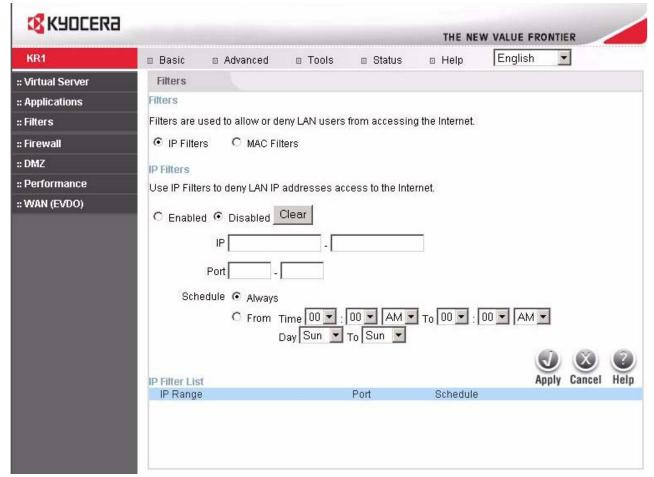
Filters - Filters are used to deny or allow LAN (Local Area Network) computers from accessing the Internet. The
