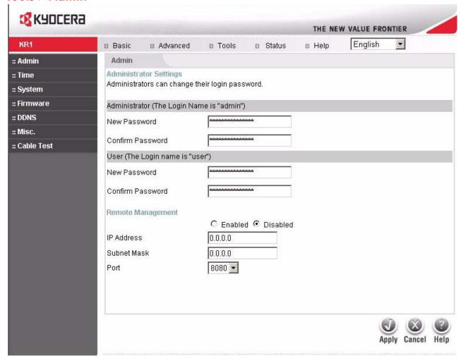
The **Tools > Admin** menu allows an administrator to change the system password. Two account options are available: **admin** and **user**. The **Admin** account option allows read/write access. The **User** account option allows for read-only access only. Within this option, the user can view settings, but cannot make any changes.
