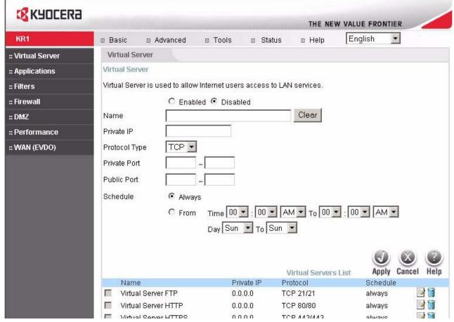
The Kyocera KR1 Mobile Router can be configured as a virtual server so that remote users accessing Web or FTP services via the public IP address can be automatically redirected to local servers in the LAN (Local Area Network).
