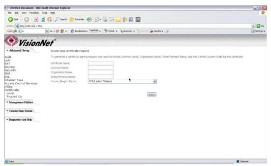
Figure 50. Advanced Setup – Local – Create Certificate
