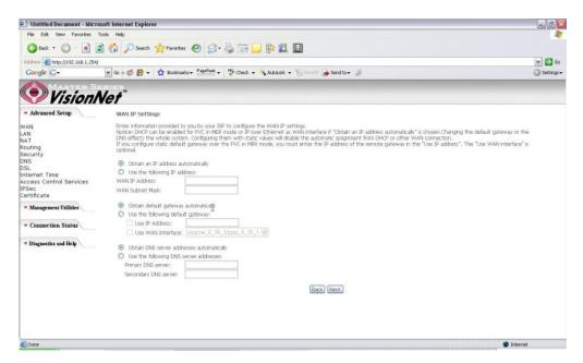
Figure 11. Quick Setup – WAN IP Settings
