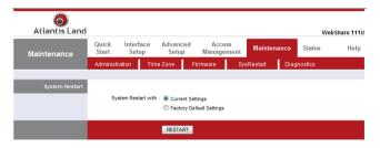
If you wish to restart the router using the factory default settings (for example, after a firmware upgrade or if you have saved an incorrect configuration), select **Factory Default Settings** to reset to factory default settings.
