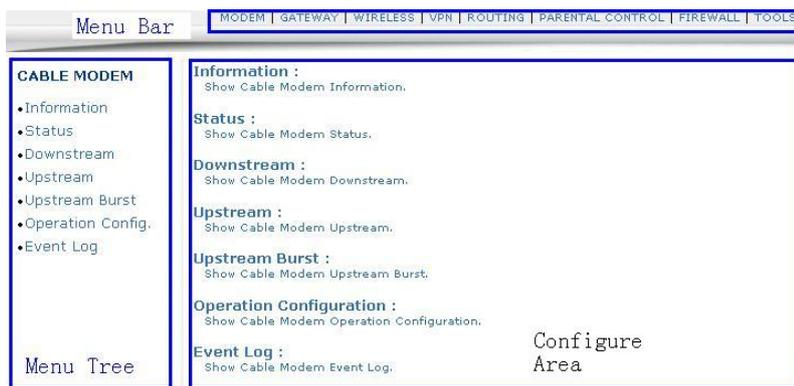
Menu Bar includes top level menu, like GATEWAY, WIRELESS and VPN. Once user select the option in menu bar, Menu Tree will be changed correspondently. To change parameter settings, user needs to operate in Configure Area.
