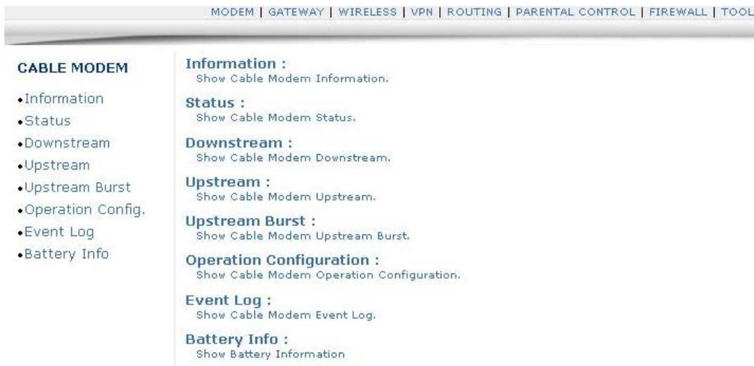
Menu Bar includes top level menu, like GATEWAY, WIRELESS and VPN. Once user select the option in menu bar, Menu Tree will be changed correspondently. To change parameter settings, user needs to operate in Configure Area. Below chapter is to go through page by page, to ensure that you're clear about each feature and how to use it.
