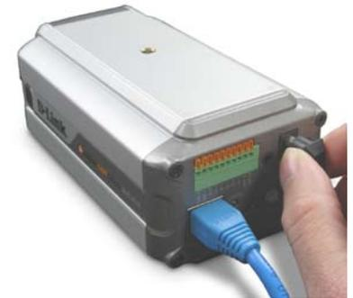
**Note:** When you have a proper connection, the LED will turn green. The light may cycle on and off and your computer may show an intermittent loss of connectivity, this is normal until you have configured your Network Camera.
