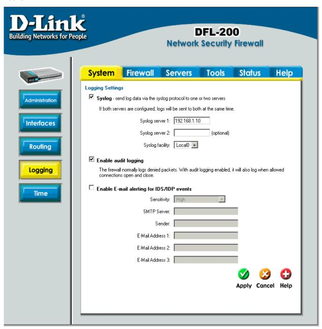
All logging is done to Syslog recipients. The log format used for syslog logging is suitable for automated processing and searching.
