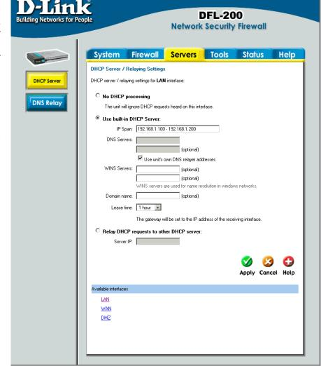
Server assigns and manages IP addresses from specified address pools within the firewall to the DHCP clients.
