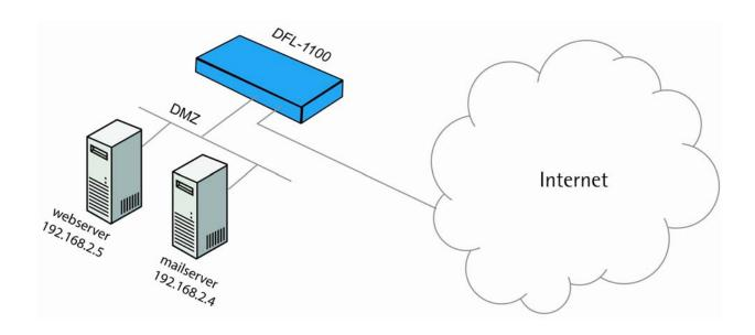
Intrusion detection and prevention can be enabled for both policies and port mappings. In this example we are using a port mapping. The policy setup is quite similar.
