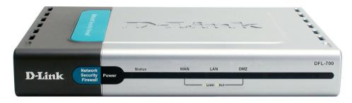
Power: A solid light indicates a proper connection to the power supply.
