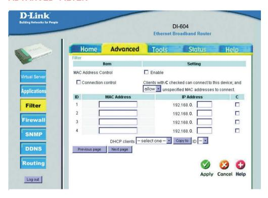
**MAC Address Control** allows you to assign different access rights for different users and to assign a specific IP address to a certain MAC address.
