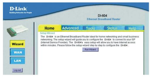
The Setup Wizard page is the first page that appears when logging into the web-based management interface. The Setup Wizard is a utility used to quickly configure the DI-604. It will guide you through three quick and basic steps to help you connect to your ISP. You will be connected to your ISP (Internet Service Provider) and have Internet access within minutes.
