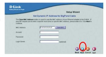
address, please enter it in. The CLONE MAC Address button is used to copy the MAC address of your Ethernet adapter to the DI-604 WAN interface. Click **Next**
