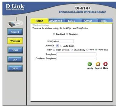
Wi-Fi Protected Access - Pre-Shared Key mode means that the wireless client and the router must have the same passphrase in order to establish the wireless connection. A RADIUS server is **not** required with PSK.
