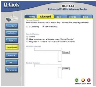
Use Domain filters to allow or deny computers access to specific Internet domains whether it is through www, ftp, SNMP, etc. Domain filters apply to both wired computers connected to one of the four Ethernet LAN ports and to wireless clients connected wirelessly to the DI-614+.
