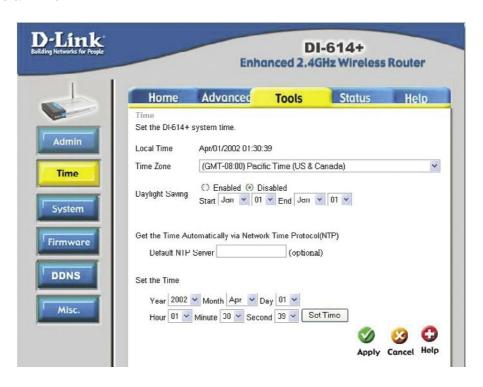
Set the time here by entering it manually or by using NTP (Network Time Protocol.) NTP is a standard protocol on the Internet that sychronizes the time settings accurately for all the computers on your network.
