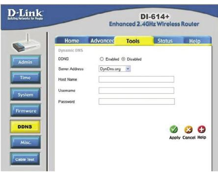
DDNS (Dynamic Domain Name System) keeps dynamic IP addresses (e.g., IP addresses assigned by a DHCP capable router or server) linked to a domain name. Users who have a Dynamic DNS account may use this feature on the DI-614+.
