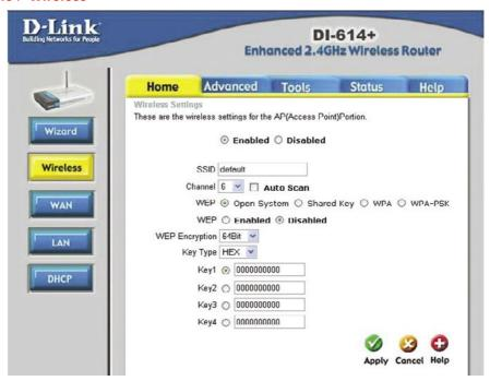
Wireless Settings are settings for the (Access Point) Portion of the Wireless Router. It allows you to change the wireless settings to fit an existing wireless network or to customize your wireless network.
