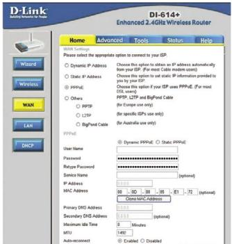
Most DSL users will select this option to obtain an IP address automatically from their ISP through the use of PPPoE.
