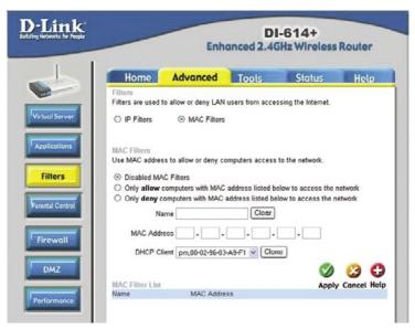
MAC (Media Access Control) Filters are used to deny or allow LAN (Local Area Network) computers from accessing the Internet and network by their MAC address.
