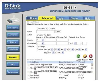
Firewall Rules is an advance feature used to deny or allow traffic from passing through the device. It works in the same way as IP Filters with additional settings. You can create more detailed rules for the device.
