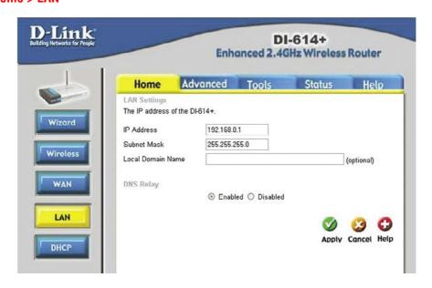
**LAN** is short for Local Area Network. This is considered your internal network. These are the IP settings of the LAN interface for the DI-614+. These settings may be referred to as Private settings. You may change the LAN IP address if needed. The LAN IP address is private to your internal network and cannot be seen on the Internet.
