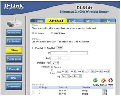
Use IP (Internet Protocol) filters to allow or deny computers access to the Internet based on their IP address.
