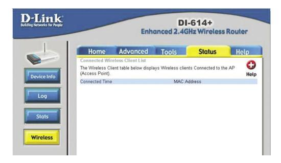
The wireless client table displays a list of current connected wireless clients. This table also displays the time and MAC address of the wireless client connected.
