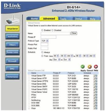
The DI-614+ can be configured as a virtual server so that remote users accessing Web or FTP services via the public IP address can be automatically redirected to local servers in the LAN (Local Area Network).
