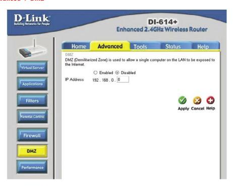
If you have a computer that cannot run Internet applications properly from behind the DI-614+, then you can allow that computer to have unrestricted Internet access. Enter the IP address of that computer as a DMZ (Demilitarized Zone) host with unrestricted Internet access. Adding a client to the DMZ may expose that computer to a variety of security risks, so only use this option as a last resort.
