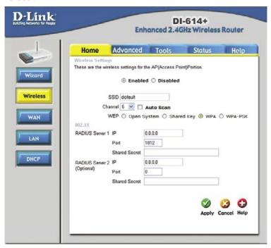
Wi-Fi Protected Access authorizes and authenticates users onto the wireless network. WPA uses stronger security than WEP and is based on a key that changes automatically at a regular interval. This mode requires a RADIUS server in the network.
