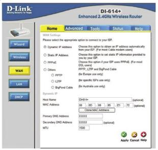
Most Cable modem users will select this option to obtain an IP Address automatically from their ISP (Internet Service Provider).
