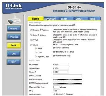
Point-to-Point Tunneling Protocol (PPTP) is a WAN connection used in Europe.
