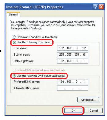
You have successfully assigned a Static IP Address.
