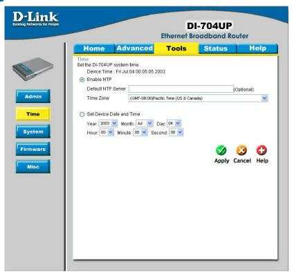
The system time is the time used by the DI-704UP for scheduling services. You can manually set the time or connect to a NTP (Network Time Protocol) server. If an NTP server is set, you will only need to set the time zone.
