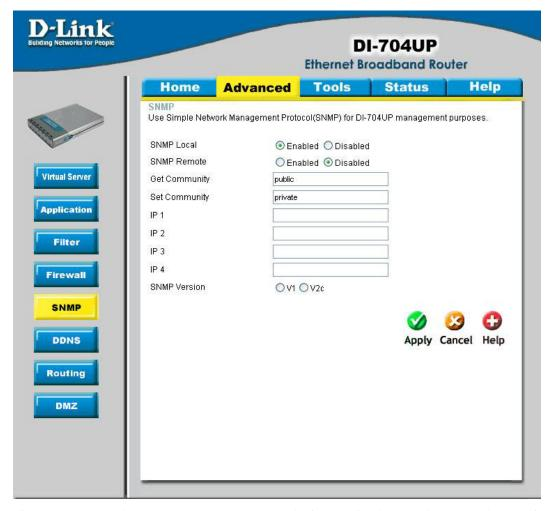
SNMP (Simple Network Management Protocol) is a widely used network monitoring and control protocol that reports activity on each network device to the administrator of the network. SNMP can be used to monitor traffic and statistics of the DI-704UP. The DI-704UP supports SNMP v1.
