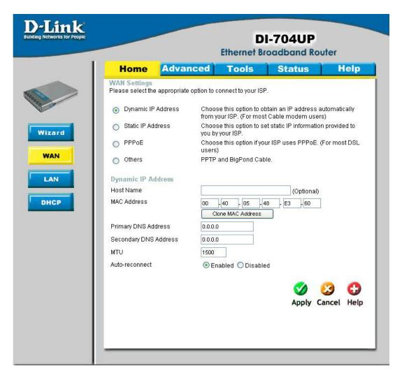
WAN is short for Wide Area Network. The WAN settings can be referred to as the Public settings. All IP information in the WAN settings are public IP addresses which are accessible on the Internet. The WAN settings consist of four options: *Dynamic IP Address*, *Static IP Address*, *PPPoE*, *and Others*. Select the appropriate option and fill in the information needed to connect to your ISP.
