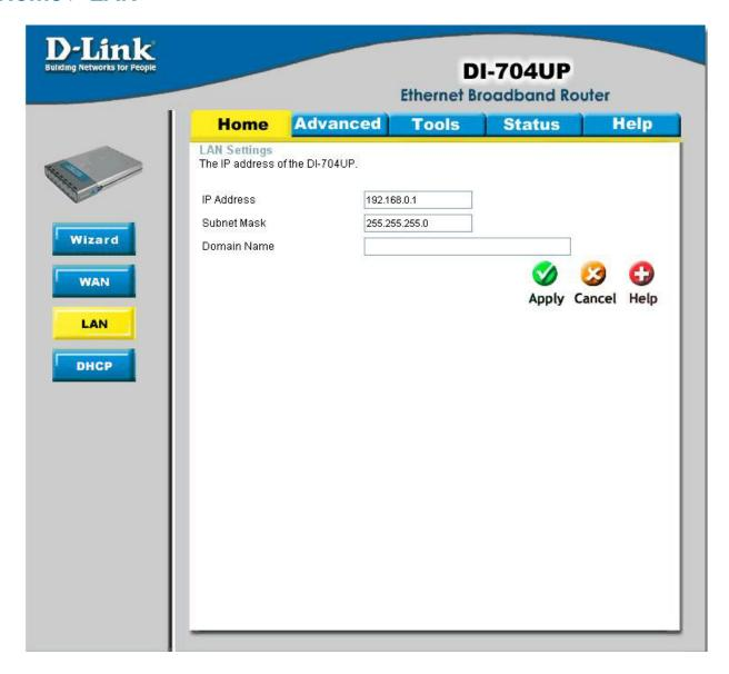
LAN is short for Local Area Network. This is considered your internal network. These are the IP settings of the LAN interface for the DI-704UP. These settings may be referred to as Private settings. You may change the LAN IP address if needed. The LAN IP address is private to your internal network and cannot be seen on the Internet.
