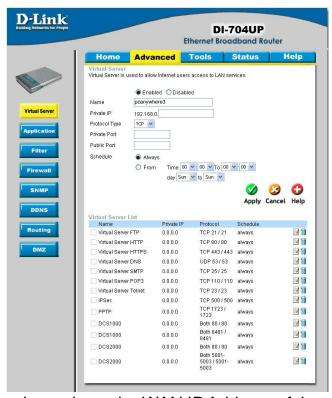
**Step 10** Run *PCAnywhere* from the remote site and use the WAN IP Address of the router, not your computer's IP Address.
