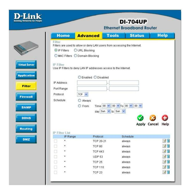
Use IP (Internet Protocol) filters to allow or deny computers access to the Internet based on their IP address.
