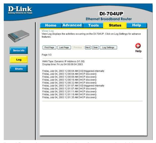
The Broadband Router keeps a running log of events and activities occurring on the router. If the device is rebooted, the logs are automatically cleared. You may save the log files under **Log Settings**.
