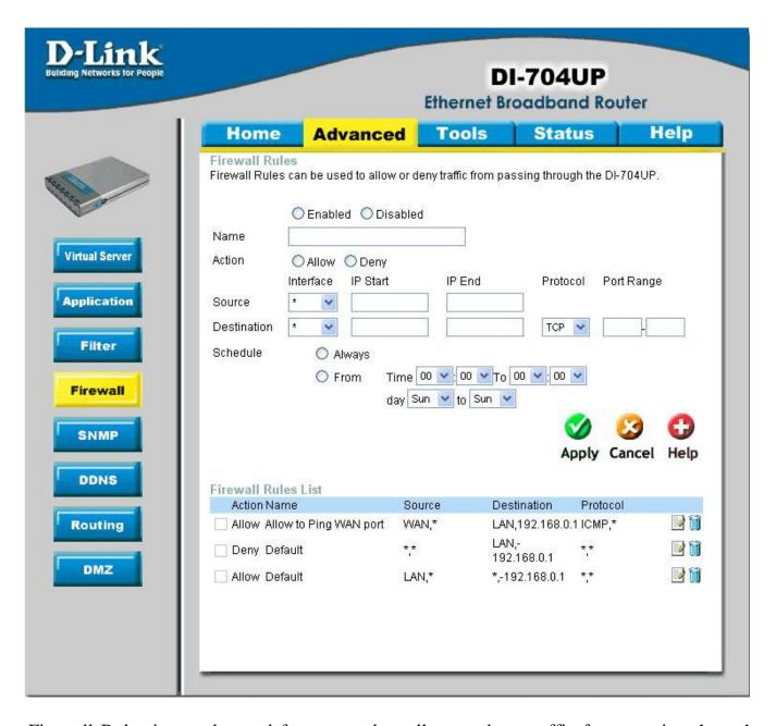
Firewall Rules is an advanced feature used to allow or deny traffic from passing through the Broadband Router. It works in the same way as IP Filters with additional settings. You can create more detailed access rules for the DI-704UP. When virtual services are created and enabled, it will also display in Firewall Rules. Firewall Rules contains all network firewall rules pertaining to IP (Internet Protocol).
