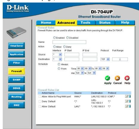
**Step 5** Select **LAN** as the **Destination** and enter the IP Address of the computer on your local network that you want to allow the incoming service to. This will not work with a range of IP Addresses.
