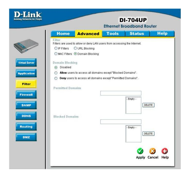
Use Domain filters to allow or deny computers access to specific Internet domains whether it is through www, ftp, snmp, etc. Domain filters apply to wired computers connected to one of the four Ethernet LAN ports to the DI-704UP.
