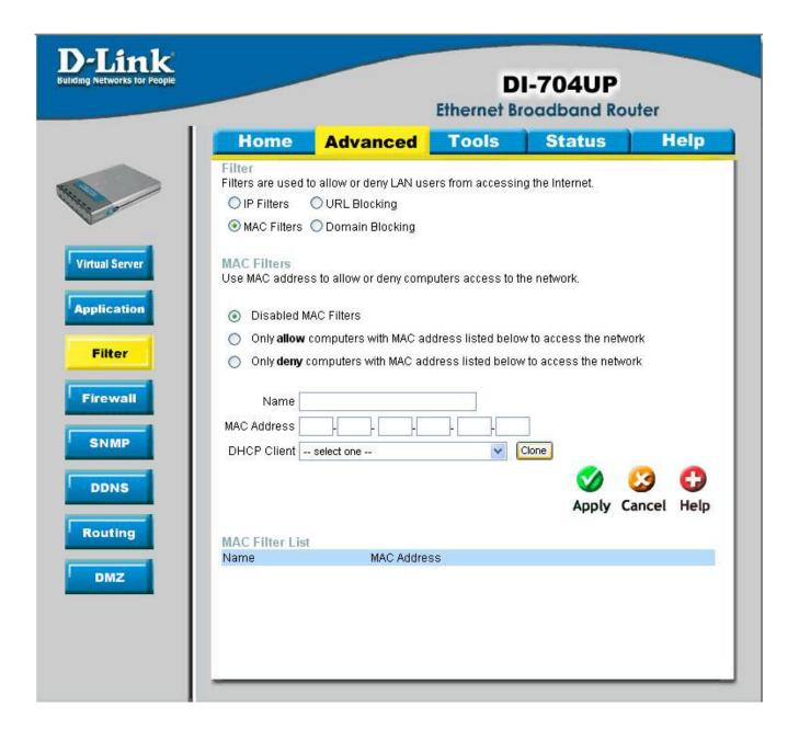
MAC (Media Access Control) Filters are used to allow or deny LAN (Local Area Network) computers from accessing the Internet and network by their MAC address.
