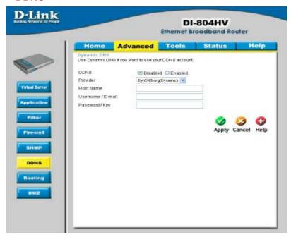
DDNS (Dynamic Domain Name System) keeps dynamic IP addresses (e.g., IP addresses assigned by a DHCP capable router or server) linked to a domain name. Users who have a Dynamic DNS account may use this feature on the DI-804HV.
