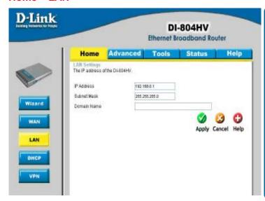
LAN (Local Area Network). This is considered your internal network. These are the IP settings of the LAN interface for the DI-804HV. These settings may be referred to as Private settings. You may change the LAN IP address if needed. The LAN IP address is private to your internal network and cannot be seen on the Internet.
