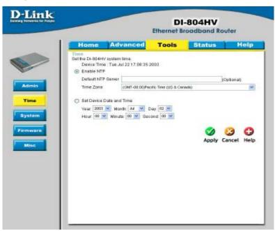
Set the time here by entering it manually or use NTP (Network Time Protocol.) NTP is standard protocol on the Internet that synchronizes the time settings accurately for the DI-804HV.
