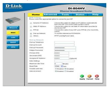
Most Dial-up users will select this option to connect to their ISP through an analog dial-up modem. This feature can be used as a back-up when your broadband connectivity is unavailable.
