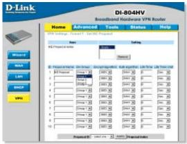
**Step 9** Select DES or 3DES as the Encryption Algorithm and either SHA-1 or MD5 as the Authentication Algorithm.
