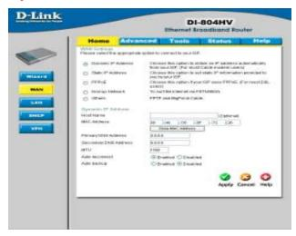
Most Cable modem users will select this option to obtain an IP Address automatically from their ISP (Internet Service Provider).
