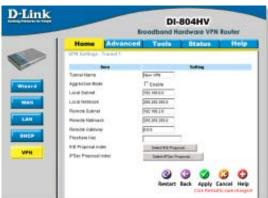
**Step 6** In the Remote Gateway field enter the WAN IP address of the remote DI-804HV and in the Preshared Key field, enter a key which must be exactly the same as the Preshared Key that is configured on the remote DI-804HV.
