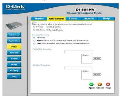
Use Domain Blocking to allow or deny computers access to specific Internet domains whether it is through www, ftp, snmp, etc.
