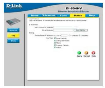
The DI-804HV can be set up to send the log files to a specific E-Mail Alertemail address.
