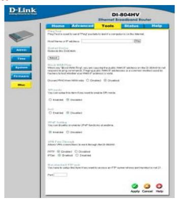
Ping Test- In the open box, enter an URL (i.e. www.dlink.com) or an IP address and click on Ping to test your internet connection.
