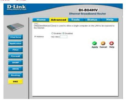
If you have a computer that cannot run Internet applications properly from behind the DI-804HV, then you can allow that computer to have unrestricted Internet access. Enter the IP address of that computer as a DMZ (Demilitarized Zone) host with unrestricted Internet access. Adding a client to the DMZ may expose that computer to a variety of security risks; so only use this option as a last resort.
