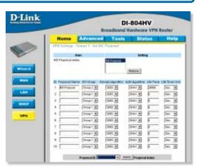
**Step 15** Select 3DES as the Encryption Algorithm and MD5 as the Authentication Algorithm.
