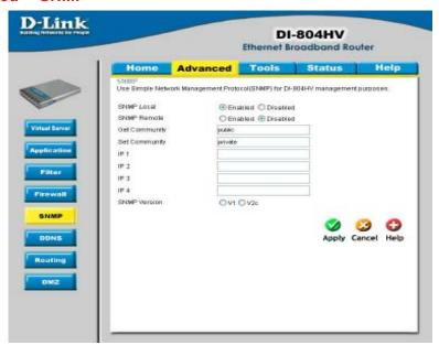
SNMP (Simple Network Management Protocol) is a widely used network monitoring and control protocol that reports activity on each network device to the administrator of the network. SNMP can be used to monitor traffic and statistics of the DI-804HV. The DI-804HV supports SNMP v1 or v2c
