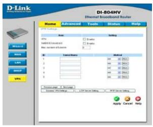
**VPN Settings** are settings that are used to create virtual private tunnels to remote VPN gateways. The tunnel technology supports data confidentiality, data origin, authentication and data integrity of network information by utilizing encapsulation protocols, encryption algorithms, and hashing algorithms.
