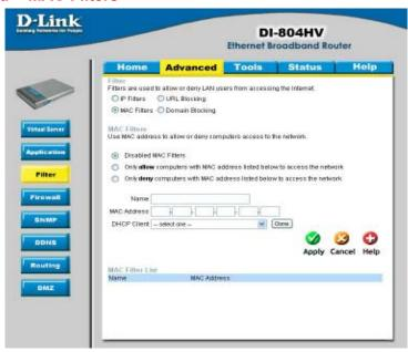
MAC (Media Access Control) Filters are used to deny or allow LAN (Local Area Network) computers from accessing the Internet and network by their MAC address.
