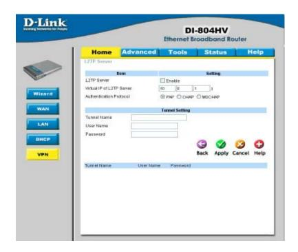
Enable L2TP Server-Click to enable the L2TP Server function.
