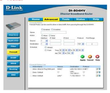
Firewall Rules is an advance feature used to deny or allow traffic from passing through the device. It works in the same way as IP Filters with additional settings. You can create more detailed rules for the device.
