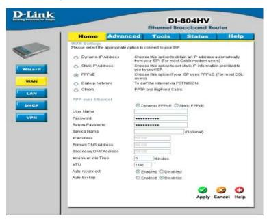
Most DSL users will select this option to obtain an IP address automatically from their ISP through the use of PPPoE.
