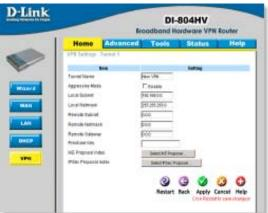
**Step 5** In the Remote Subnet and Remote Netmask fields enter the network identifier for the DI-804V's LAN and the corresponding subnet mask.
