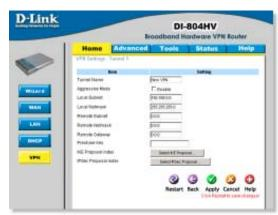
**Step 5** In the Remote Subnet and Remote Netmask fields enter the network identifier for the remote DI-804HV's LAN and the corresponding subnet mask.
