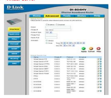
The DI-804HV can be configured as a virtual server so that remote users accessing Web or FTP services via the public IP address can be automatically redirected to local servers in the LAN (Local Area Network).
