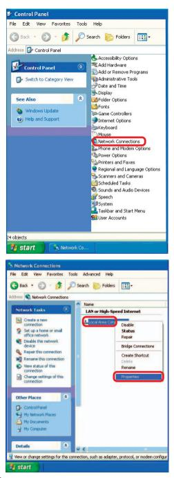
Assigning a Static IP Address in Windows XP/2000
