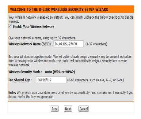
On this page, you can check the **Wireless Status, Network Name (SSID), Wireless Security Mode,** and **Pre-shared Key**.
