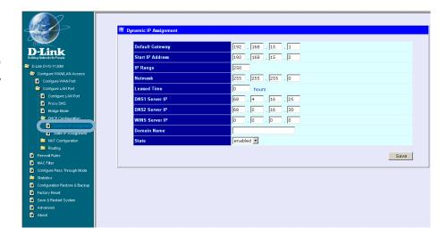
**Default Gateway -** This specifies the Gateway IP Address that will be assigned to and used by the DHCP clients.
