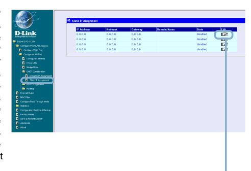
Click the edit icon on the window above to access the second **Static IP Assignment** window:
