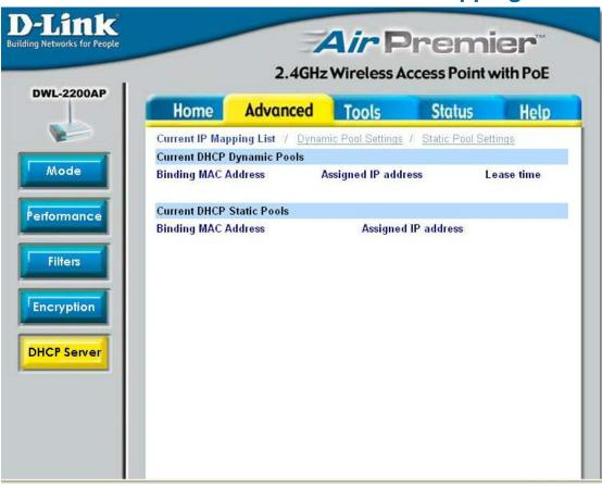
This screen displays information about the current DHCP dynamic and static IP address pools. This information is available when you enable the DHCP function of the DWL-2200AP and assign dynamic and static IP address pools.
