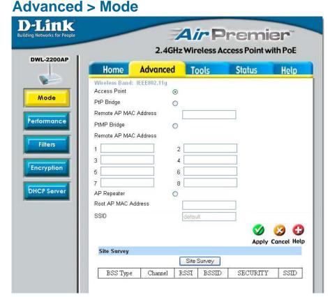
**PtMP Bridge -** Allows you to connect multiple wireless LANs together. Other wireless LANs must be using DWL-2200APs. Click to enable, and enter up to 8 remote AP MAC addresses.
