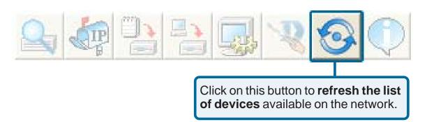
Devices with a checkmark next to them are still available on the network. Devices with an X are no longer available on the network.
