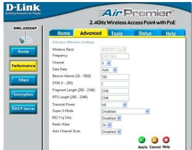
Beacon Interval- Beacons are packets sent by an access point to synchronize a
