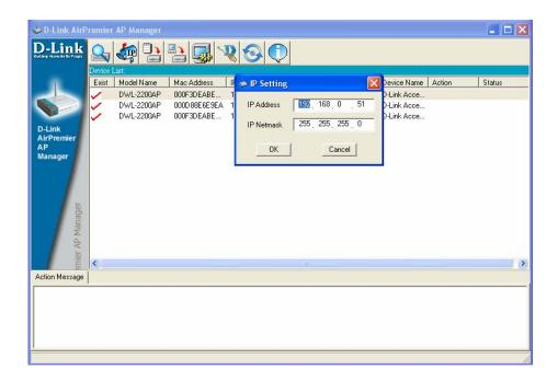
Select the AP that you want to assign an IP address and click the IP button. Enter the IP Address and IP Netmask for the selected device and click OK.
