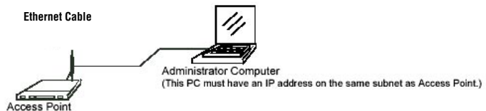
ETHERNET CONNECTIONS WHEN USING STATIC IP FOR INITIAL CONFIGURATION
