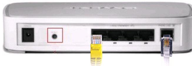
5. Connect the power adapter to the Modem's Power Port and the other end, plug into an Electrical Power Point. Switch on the modem.
