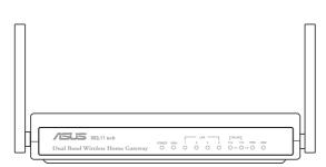
The **SpaceLink<sup>™</sup> Dual-Band Home Gateway (WL-600)** creates a wireless network using the IEEE 802.11b and 802.11a wireless standards and allows sharing a single Internet connection.
