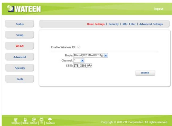
The screenshot shows the WATEEN modem setup interface. At the top, there is a green header with the WATEEN logo and a 'logout' link. Below the header, there is a navigation menu with buttons for 'Status', 'Setup', 'WLAN', 'Advanced', 'Security', and 'Tools'. The 'WLAN' button is highlighted in red. The main content area is titled 'Basic Settings | Security | MAC Filter | Advanced Settings'. It contains the following configuration options:
