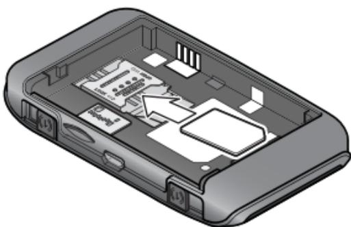
2. Insert the battery as shown in the illustration. (The battery installs easily. If it does not go in easily, check the orientation. Do not force it.)
