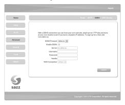
DDNS is a dynamic domain analysis system. After applying DDNS, a dynamic IP address to the mainframe also can provide domain name services. For example, the mainframe through dial-up or XDSL DHCP server gets IP address and domain names dynamically. Enable and configure DDNS so the host's IP address changes will not affect the users who visit through the domain name.
