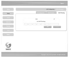
You can set MAC address and IP address binding, create a DHCP binding table to mapping MAC address and IP address of clients. When DHCP
