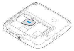
3. Insert the SIM card into the slot until it is fully inserted.
