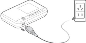
**NOTE:** The plug only fits one way to connect your device. Do not use excessive force to insert the plug.
