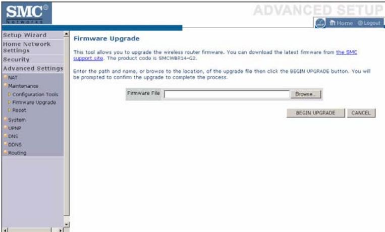
Go to [www.smc.com](http://www.smc.com) to find the latest firmware. Download the firmware to your hard drive first. Click **Browse...** to locate the saved file. After locating the new firmware file, click **BEGIN UPGRADE**. Follow the instructions to complete the upgrade. After restarting, check the Status page to make sure the device is running the new code.
