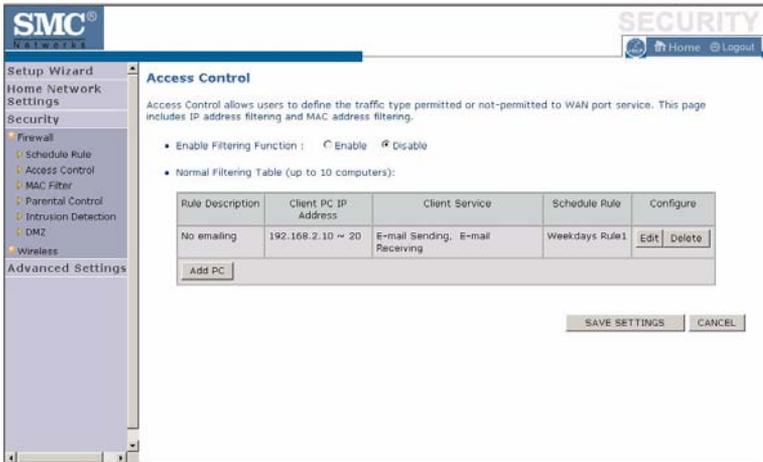
Used in conjunction with the Schedule Rule screen, the Access Control screen allows users to define the outgoing traffic permitted or not-permitted. The default is to permit all outgoing traffic.
