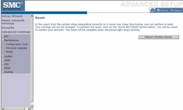
To perform a system reset, click the **Reboot Wireless Router** button in the screen above. The configurations that you have set previously will not be changed back to the factory default settings.
