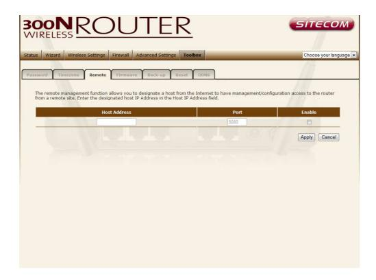
**Host Address** This is the IP address of the host in the Internet that will have management/configuration access to the Broadband router from a remote site. If the Host Address is left 0.0.0.0 this means anyone can access the router's web-based configuration from a remote location, providing they know the password.
