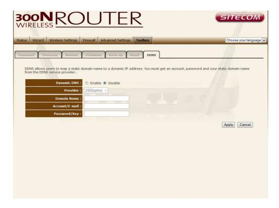
**Enable/Disable** Enable or disable the DDNS function of this router
