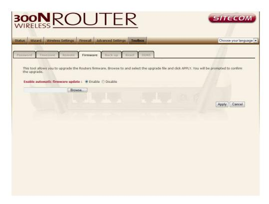
**Firmware Upgrade** This tool allows you to upgrade the Broadband router's system firmware. To upgrade the firmware of your Broadband router, you need to download the firmware file to your local hard disk, and enter that file name and path in the appropriate field on this page. You can also use the Browse button to find the firmware file on your PC.
