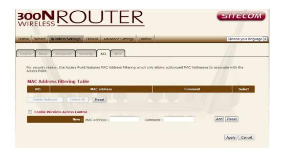
Enable wireless access control Enables the wireless access control function
