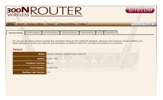
The System status section allows you to monitor the current status of your router the UP time, hardware information, serial number as well as firmware version information is displayed here.
