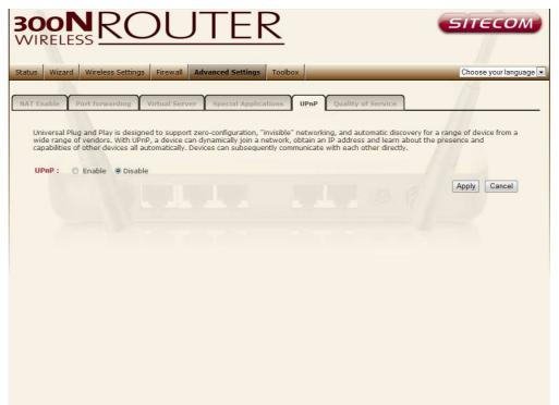
**UPnP Feature** You can enable or Disable the UPnP feature here. After you enable the UPnP feature, all client systems that support UPnP, like Windows XP, can discover this router automatically and access the Internet through this router without having to configure anything. The NAT Traversal function provided by UPnP can let applications that support UPnP connect to the internet without having to configure the virtual server sections.
