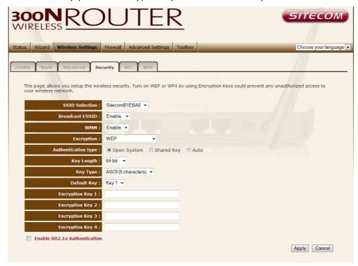
**Key Length** You can select the WEP key length for encryption, 64-bit or 128-bit. The larger the key will be the higher level of security is used, but the throughput will be lower.
