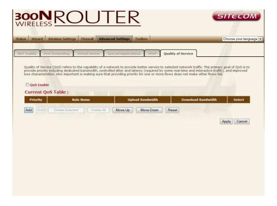
**Enable/Disable QoS** You can check "Enable QoS" to enable QoS functionality for the WAN port.
