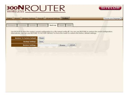
Use the "Backup" tool to save the Broadband router current configuration to a file named "**config.bin**" on your PC. You can then use the "Restore" tool to restore the saved configuration to the Broadband router. Alternatively, you can use the "Restore to Factory Defaults" tool to force the Broadband router to perform a power reset and restore the original factory settings.
