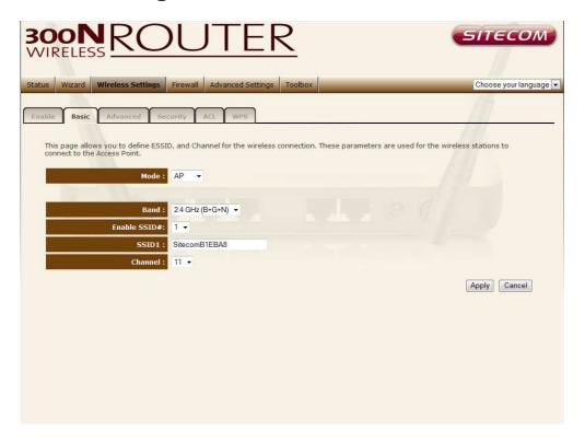
**Band** Allows you to set the AP fixed at 802.11b or 802.11g mode. You can also select B+G mode to allow 80211b and 802.11g clients at the same time.
