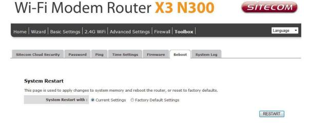
Whenever you use the Web configuration to change system settings, the changes are initially placed in temporary storage. To save your change for future use, you have to click "Apply" to reboot the router. If you have encountered problems during the configuration, you can click the "OPS" button in the top panel of the router over 15 seconds to reset default settings.
