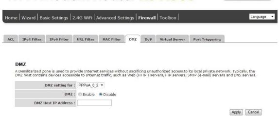
The DMZ Host is a local computer exposed to the Internet. When setting a particular internal IP Address as the DMZ Host, all incoming packets will be checked by the firewall and NAT algorithms then passed to the DMZ Host.
