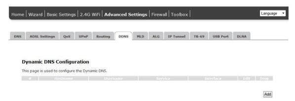
Dynamic DNS (DDNS) allows you to map the static domain name to a dynamic IP address. You must get an account, password and your static domain name from the DDNS service providers.
