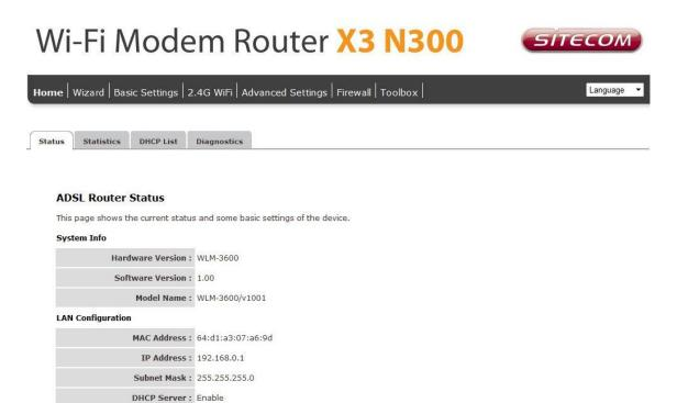
The System status section allows you to monitor the current status of your modem/router: the UP time, hardware information, serial number as well as firmware version information is displayed here. The page also shows extensive information concerning the ADSL status and current settings.
