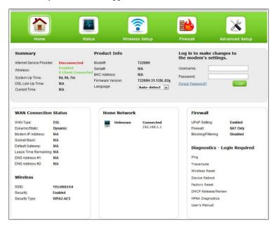
**3.** Enter the username "admin" and the password (printed on the label located on the bottom of the Gateway) in the Username and Password text boxes at the top right side of the screen, then click **Login**.
