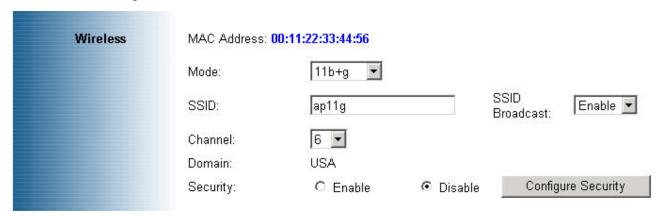
**SSID:** The service set identifier (SSID) or network name. It is case sensitive and must not exceed 32 characters, which may be any keyboard character. You shall have selected the same SSID for all the APs that will be communicating with mobile wireless stations.
