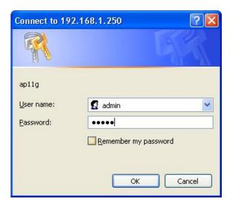
To start configure the outdoor Wireless 11g AP, you must login as "admin" in the **User Name** box. And input password "admin" on the password section.
