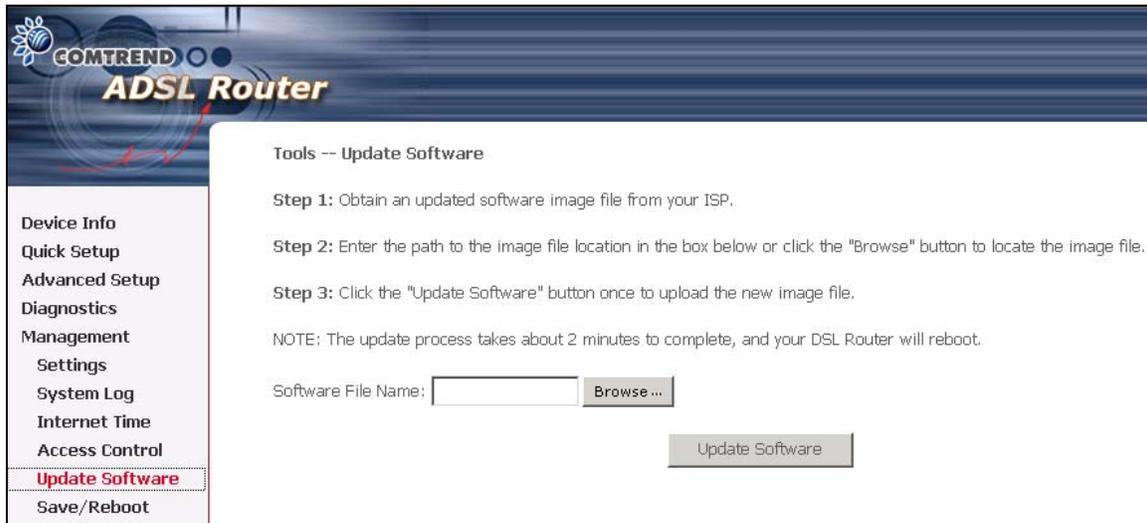
The screenshot shows the 'Update Software' screen in the Comtrend ADSL Router web interface. The left sidebar contains a navigation menu with the following items: Device Info, Quick Setup, Advanced Setup, Diagnostics, Management, Settings, System Log, Internet Time, Access Control, Update Software (highlighted in red), and Save/Reboot. The main content area is titled 'Tools -- Update Software' and contains the following instructions:
