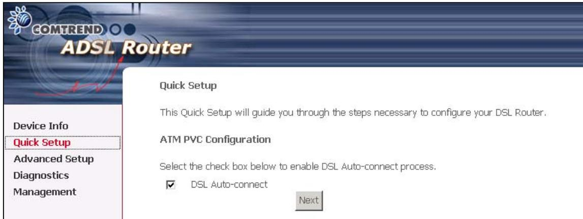
2. Click **Next** to start the setup process. Follow the online instructions to complete the setting. This procedure will skip some processes like PVC index, or encapsulation.
