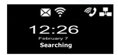
Upon inserting a SIM card, the router begins to search tor a signal from the network provider. If the signals from the network provider can not be reached, **No Service** is displayed. If the router is connected to radio access network, then the network provider name, type of radio access technology and signal strength are displayed.
