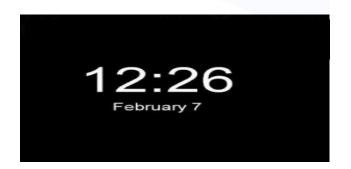
The screen automatically enters Screen Saver Mode after 60 seconds of inactivity. The Date and Time are displayed moving randomly on the screen. Short pressing the WPS key or any router state changes such as incoming VoIP call, LAN disconnect, etc. will bring the router out of Screen Saver Mode.
