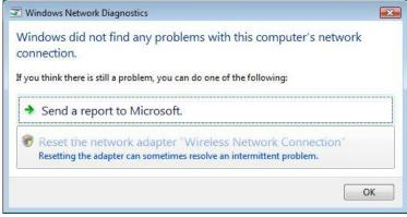
If you use Local Area Connection to connect the Router, please click Network and Sharing Center > Manage network connections > Local Area Connection > Diagnose, do the step 1 and following the message to repair it.
