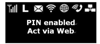
If the user has enabled the PIN security protection on the SIM card, the screen directs the user to access **4G LTE > PIN Verification** via the web interface before proceeding to use the Internet connectivity features of
