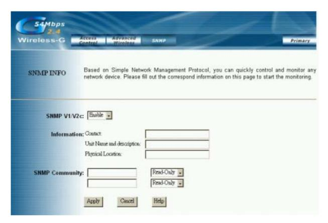
**SNMP INFO:** The SNMP screen allows you to customize the Simple Network Management Protocol (SNMP) settings. SNMP is a popular network monitoring and management protocol.
