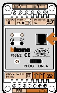
To program the telephone actuator move selector switch (3) to "PROG" and type the commands on the telephone connected to the connector (4). The programming cable is supplied.
