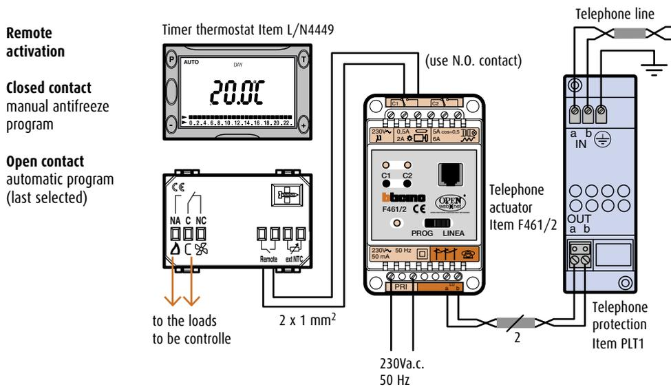
**DIAGRAM 3 CONNECTION TO THE TELEPHONE SWITCHBOARD AS AN EXTENSION**
