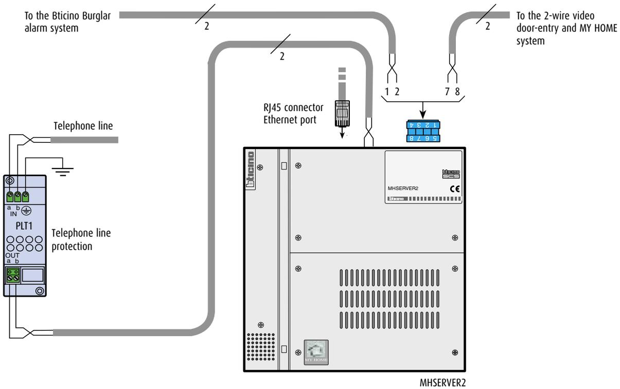
**DIAGRAM 3 CONNECTION TO THE TELEPHONE LINE AND TO THE BURGLAR ALARM CONTROL UNIT WITH DIALLING DEVICE ITEM 3500/3500N/3500GSM OR TO THE TELEPHONE DIALLING DEVICE ITEM 4075N**
