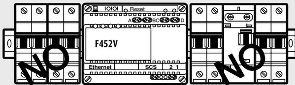
Do not move devices which may cause electromagnetic interferences close to the WEB Server video
