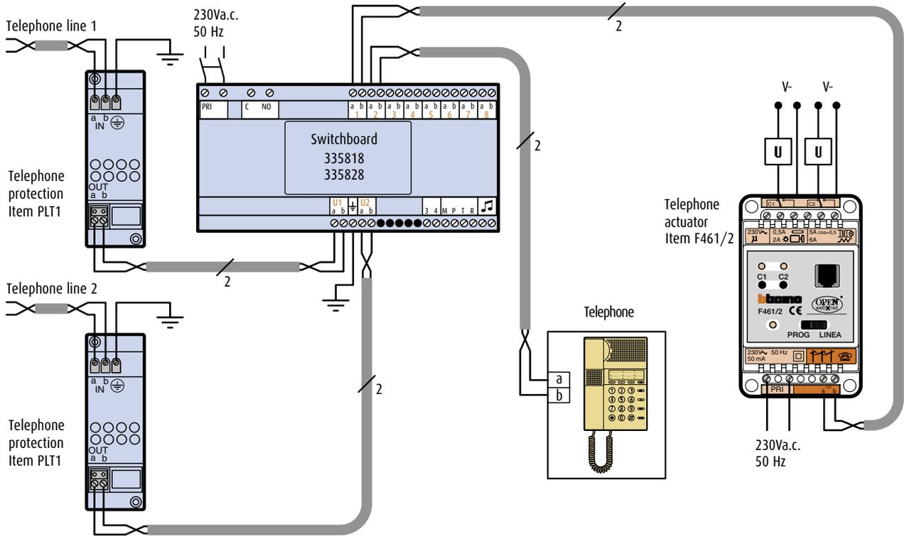
**DIAGRAM 4 DIRECT CONNECTION TO THE TELEPHONE LINE WITH MORE ACTUATORS**
