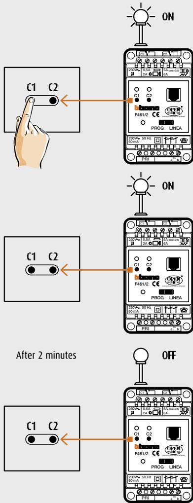
Garden lighting, "lighting" mode and "switch on-switch off" operation (bistable relay)
