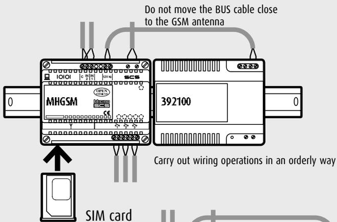
Do not move the BUS cable close to the GSM antenna
