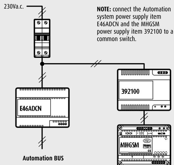
**NOTE:** connect the Automation system power supply item E46ADCN and the MHGSM power supply item 392100 to a common switch.
