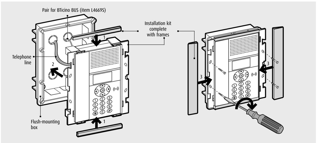
After establishing the exact point where the dialling device must be installed set up the system; trunking for the passage of the cables for BUS and telephone system, flush-mounting box and any finishings if installed in MULTIBOX switchboards.
