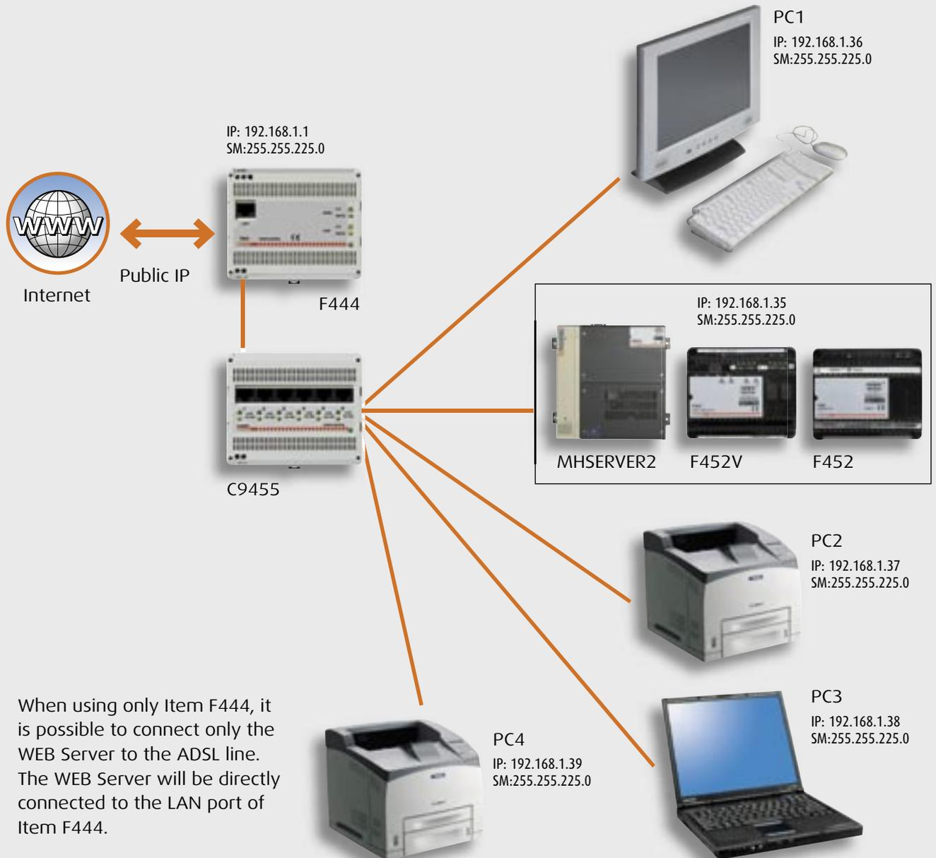
When using only Item F444, it is possible to connect only the WEB Server to the ADSL line. The WEB Server will be directly connected to the LAN port of Item F444.
