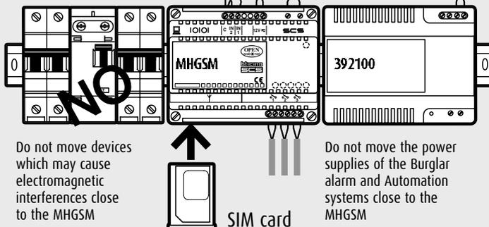
Do not move devices which may cause electromagnetic interferences close to the MHGSM
