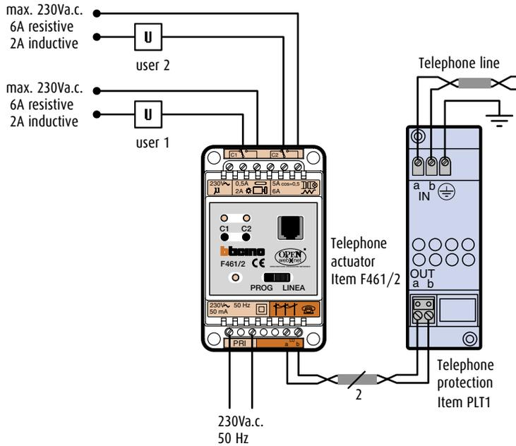
**DIAGRAM 2** CONNECTION TO THE TELEPHONE LINE SUPPLIED WITH THE BTICINO TIMER THERMOSTAT ITEM L4449/N4449
