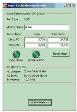
The system tray icon (and the **Status** and **Activity** buttons) can be one of three colors, indicating the modem's connection status.
