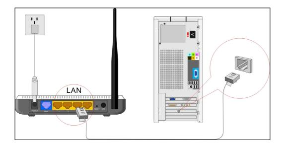
3. Connect your xDSL / cable modem to the **WAN** port of ZSR4154WE by Ethernet cable.
