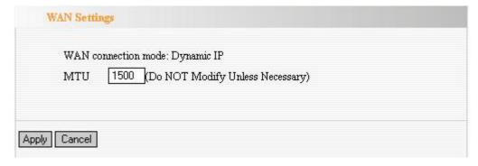
• **MTU:** Maximum Transmission Unit. It is the size of largest datagram that can be sent over a network. The default value is 1500. Do NOT modify it unless necessary.
