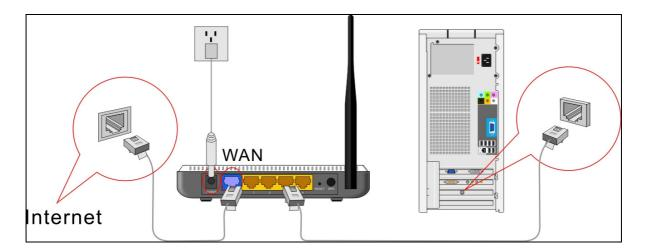
4. Please check all LEDs on the top panel. POWER LED should be steadily on, WAN and LAN LEDs should be on if the computer / network device connected to the respective port of ZSR4154WE is powered on and correctly connected. If any LED you expected is not on, please recheck the cabling, or jump to "Troubleshooting" for possible reasons and solution.
