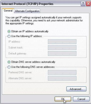
5. Or select *Use the following IP address* and enter the IP address, Subnet mask, Default gateway. Of course, you need to input the DNS server address provided by your ISP. Otherwise, you can use the ZSR4154WE's default gateway as the DNS proxy server. Click *OK* to save the configurations.
