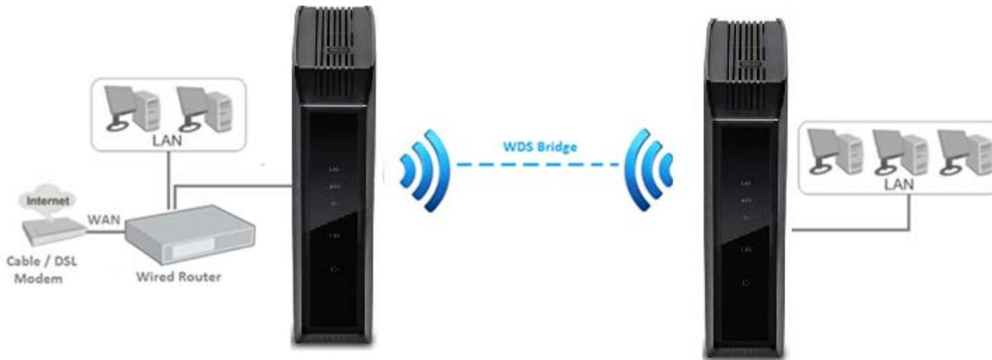
The diagram below illustrates an example of multiple WDS wireless bridge links.
